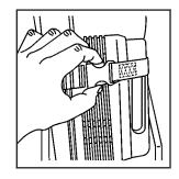
Remove the tire inflator kit strap by squeezing the two tabs of the quick release buckle.
